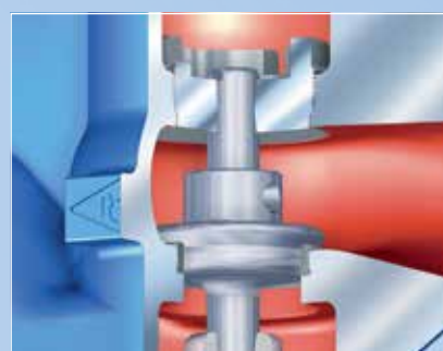
Thermal opening valve (for cooling systems) opens when the temperature at the sensor rises
