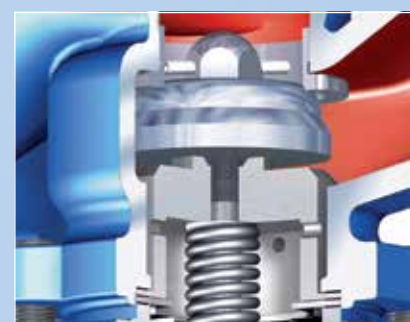
Thermal closing valve (for heating systems) closes when the temperature at the sensor rises
