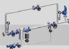
e.g. pressure reducing station PREsys®
