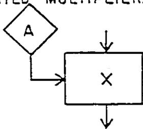
13 HIGH LIMITING OF A SIGNAL BY A MANUAL ADJUSTMENT
