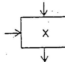
9 MULTIPLYING ONE SIGNAL BY A MANUALLY ADJUSTED MULTIPLIER.
