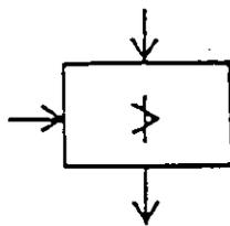
16 MANUAL TRANSFER TO OR FROM A MANUALLY ADJUSTED SIGNAL. (MANUAL-AUTOMATIC CONTROL STATION)
