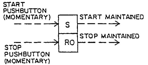
IF BOTH THE START AND STOP PUSH-BUTTONS ARE DEPRESSED, ONLY THE RESET OUTPUT IS "TRUE" OR "ON."
