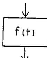
SIGNAL MODIFIED BY A FUNCTION OF TIME.
