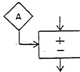
11 NON-LINEAR FUNCTION PERFORMED ON A SIGNAL
