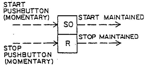
IF BOTH THE START AND STOP PUSH-BUTTONS ARE DEPRESSED, ONLY THE SET OUTPUT IS "TRUE" OR "ON."
