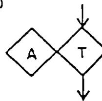
17 MANUAL TRANSFER TO OR FROM A MANUALLY ADJUSTED SIGNAL AND INCLUDING SET POINT.
