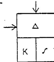
INTERNAL SET POINT TO BE DIAGRAMMED AS IN EXAMPLE 5
